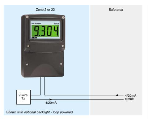
The BA304NE loop powered 4/20mA indicator is a fourth generation field mounting instrument that is mechanically compatible and electrically similar to the earlier BA304ND. It has a much larger full 4 digit display and guaranteed performance between -40 and +70°C. Like it's predecessor, the BA304NE is housed in a robust IP66 enclosure with a separate terminal compartment.
